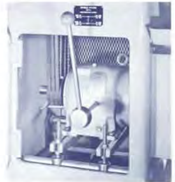
Inside view of optional geared motor drive with external shifting lever.
