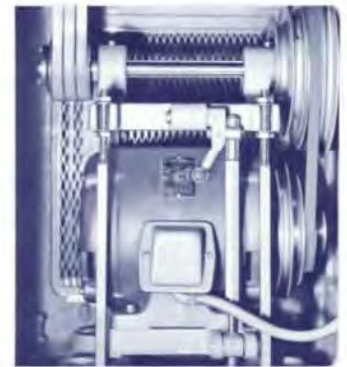
Inside view of standard, manual shift, all V-belt drive.
