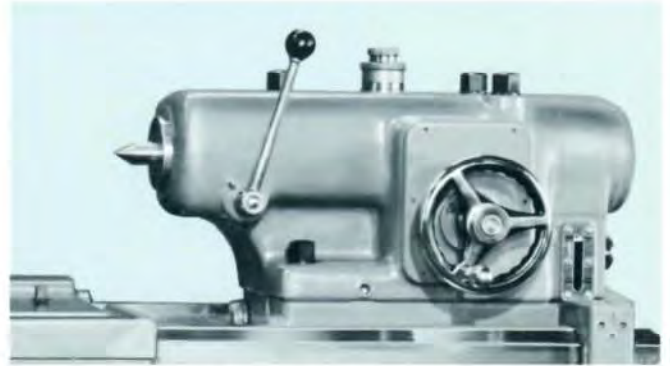
Optional combination stationary/live center in 4" diameter spindle is protected by thrust plate against binding caused by workpiece expansion. Spindle is provided with tang slot. Note graduated dial on top.
